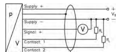
**NOTE** For the electrical connection a shielded and twisted multicore cable is recommended.
