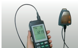
Inspection of transmitters with 4 to 20 mA interface
