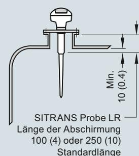
SITRANS Probe LR Einbau, Maße in mm (inch)
