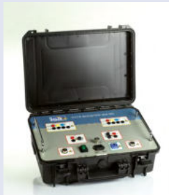
20A DC BOOSTER FOR WINDING RESISTANCE TEST
