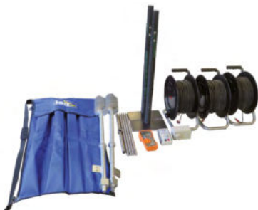
GROUND GRID TEST ACCESSORIES KIT
