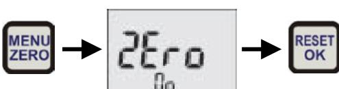
This initiates the zero point correction. The ACT (actual) value is indicated in the display as 0.0 bar. The correction remains active until the device is turned off.
