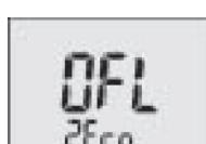
OFL/Zero is displayed for 3 seconds if the measured pressure (0 bar) is greater than 5% of the measurement range.
