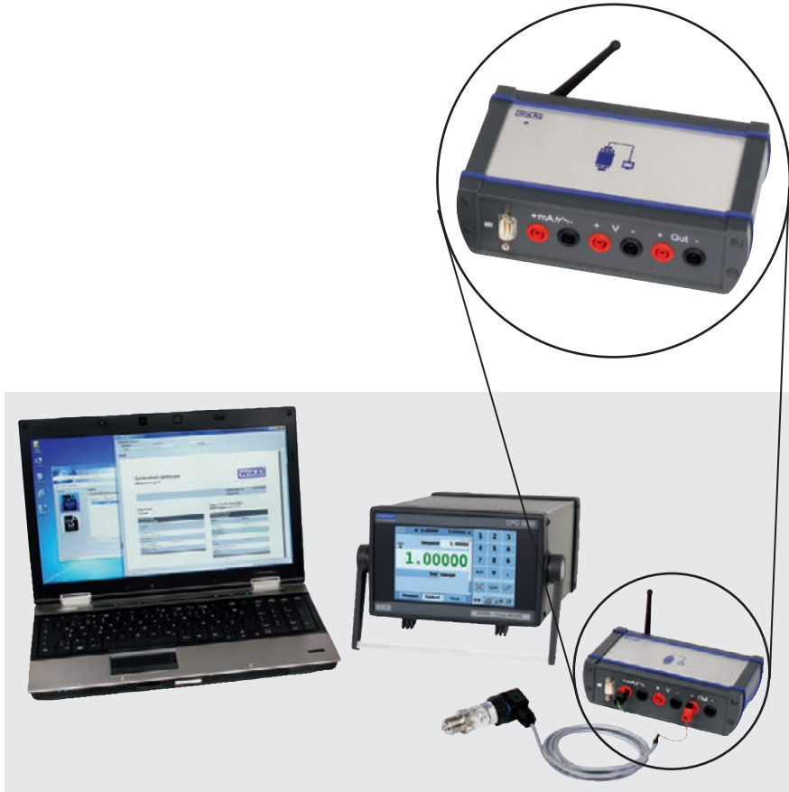
Measuring assembly: model CPC3000 high-speed pneumatic pressure controller, model CPU6000-M digital multimeter and PC/laptop
