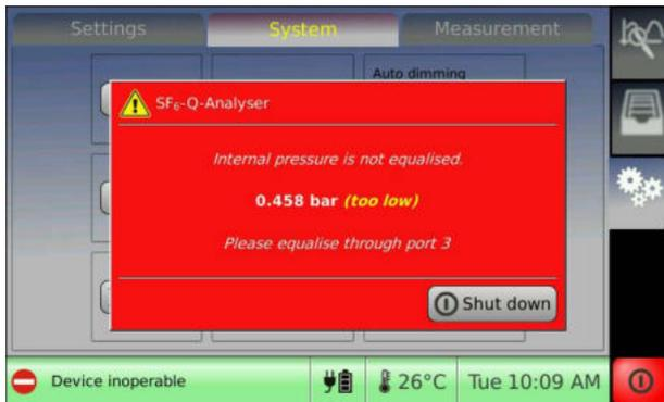
For pressure compensation, connect a gas recovery bag with the desired gas (under atmospheric pressure, max. 1,200 mbar) to the outlet for the gas recovery bag ③.
