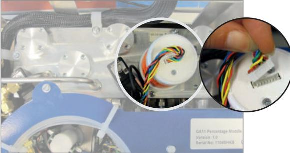
3. Screw out the sensor counterclockwise.
