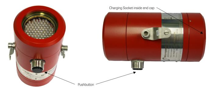
The picture above shows the FGard SIM flame simulator. The on/off pushbutton is shown to the underside of the flame simulator. The charging socket is on the reverse end from the faceplate window, inside the end cap. The FGard SIM flame simulator will operate for a maximum of 60 seconds before timing out.
